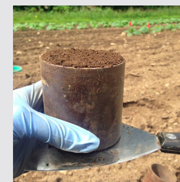
Figure 23. Bulk density soil sampler ring with intact soil core inside. (Image credit: Zineb, 2016)
