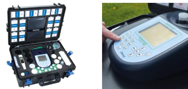
Figure 16. SKW500 Complete Soil Kit (left) and direct-reading, waterproof photometer – Soiltest 10 (right) uses battery-powered instruments to test soil pH, electrical conductivity, macronutrients and micronutrients. The kit offers an economical and simple test solution which is ideally suited to field testing. (Image credit: Palintest, 2021)
