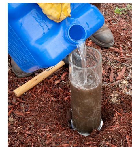
Figure 28. Infiltrometer test. (Image credit: Mississippi Watershed Management Organization, 2019. Licensed under CC BY-NC 2.0).
