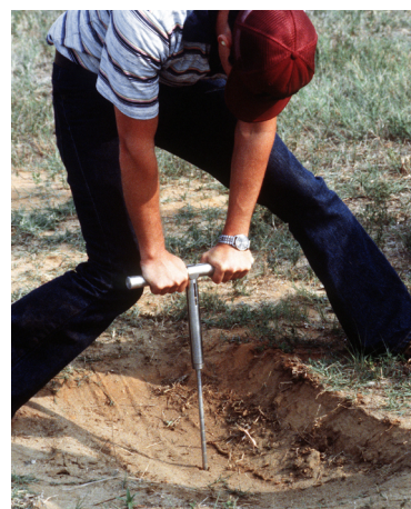
Figure 22. A penetrometer softness measurement being taken in a runway test pit. (Image credit: The U.S. National Archives, 1980)
