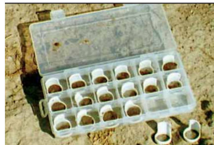
Figure 27. Plastic compartmentalized box ("soil stability kit") with 2.5cm sieves (Image credit: USDA, 1999)
